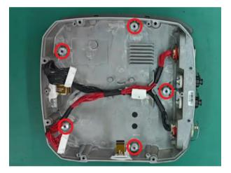
9. Place the 1.5.0 mainboard on the lower case and tighten the 5 screws.
