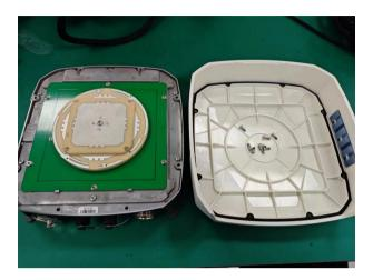
2. Unscrew the screws on the antenna and then take off the antenna.
