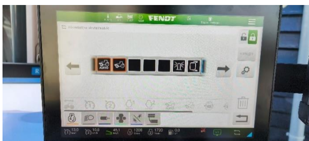
Picture 1: FendtOne Screen showing editing functions, earlier models of Fendt will have different screens
